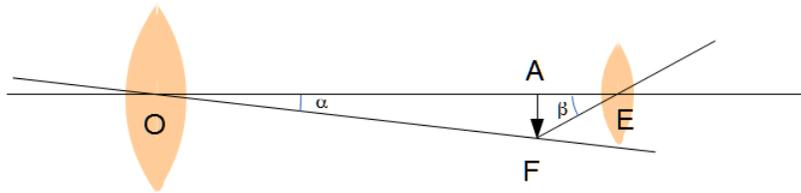
In the diagram, the image of an upright arrow (to the left of the lens O, not shown in the diagram) is formed at AF. The actual arrow subtends an angle  $\alpha$  as seen from the telescope's objective lens O, and will subtend the same angle on the focal plane, which is at a distance  $f$  (the focal length) from the lens. The size  $y = \overline{AF}$  is therefore
