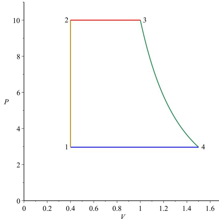
The working substance in a steam engine is, not surprisingly, steam, which is condensed to liquid water for part of the cycle. Starting at point 1, the water is in liquid form and is compressed at constant volume to a pressure  $P_2$  at point 2. Liquid water doesn't change its volume much when compressed, so the constant volume is a good approximation.
