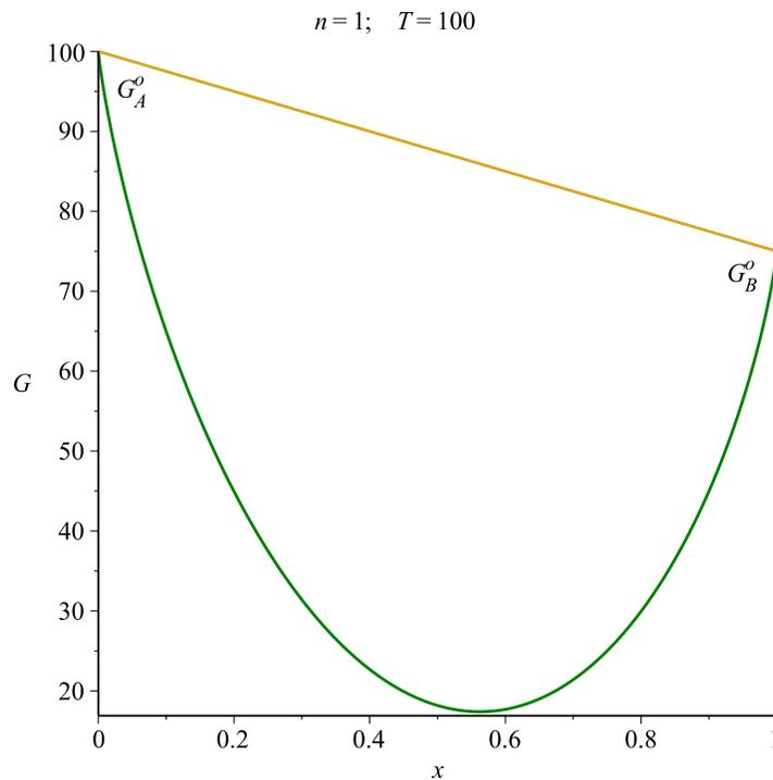
Here we've taken  $G_A^o = 100$ ,  $G_B^o = 75$ ,  $n = 1$  and  $T = 100$ . The yellow line shows the Gibbs energy from 1, where the two populations are unmixed. The green curve shows 5, where the two populations are mixed. Since the energy for the mixture is lower (because of the increase in entropy), it is the favoured state.
